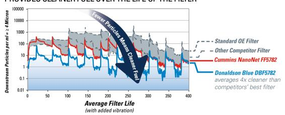
Particle retention was tested under SAE J1985 single-pass test standards with added vibration and increased particulate concentration. Test conducted March – April 2013 with a sample size of six filters per manufacturer.
