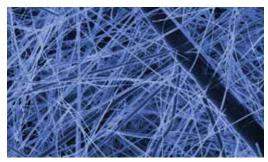
Donaldson's proprietary Synteq XP media creates small, consistent inter-fiber spacing – increasing filter capacity. These unobstructed pores result in reduced pressure drop and increased surface area for capturing and retaining more microscopic particles.
