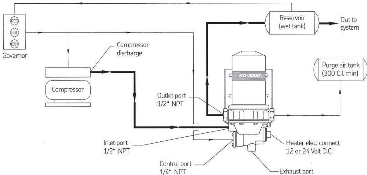
**Fig. 2** Connection schematic
