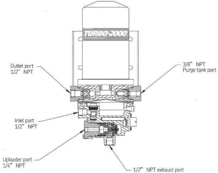
**Note: Perform all test steps, in sequence shown, to insure a properly functioning air dryer.**
