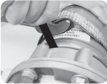
2. If above does not help, strike the cartridge with a center punch or a ball nose at the lower end where the diameter is slightly larger. This will bind together the internal components of the cartridge. Re-attempt to remove cartridge.
