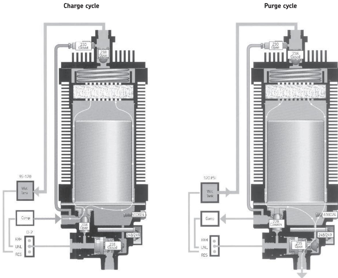
■ Clean/dry air ■ Atmospheric pressure ■ Dirty/wet charged air ■ Dirty/wet purged air
