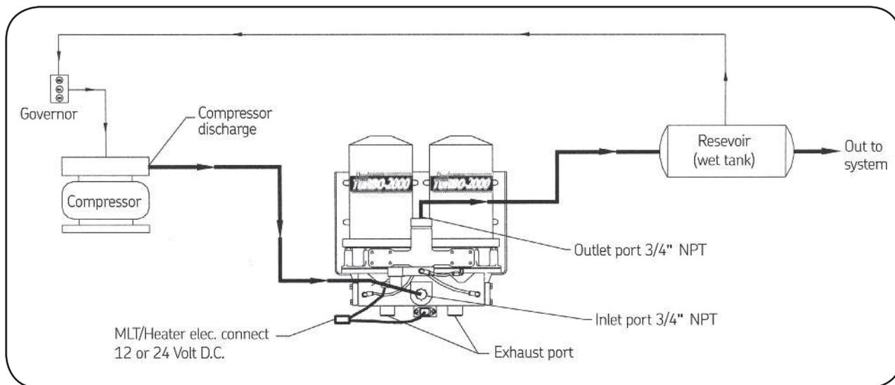
Fig. 1 Connection schematic
