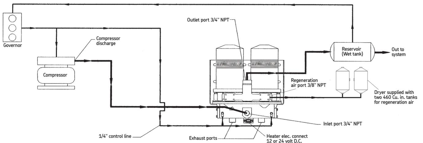
**Fig. 2** Connection schematic
