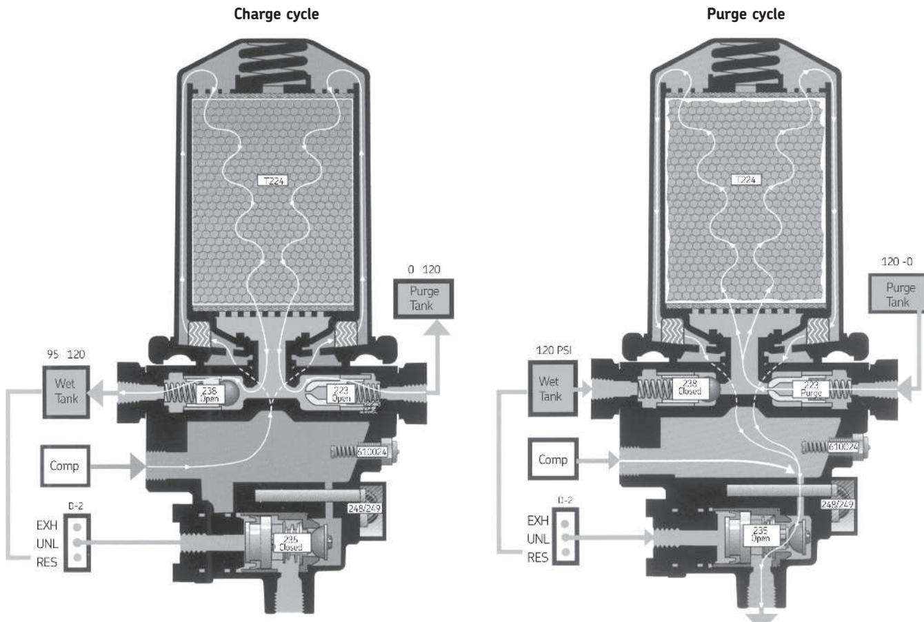
■ Clean/dry air ■ Atmospheric pressure ■ Dirty/wet charged air ■ Dirty/wet purged air
