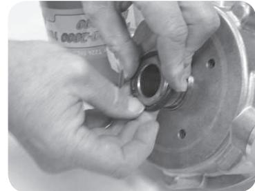
2. **Do not over-tighten** the cartridge while installing. When the rubber gasket contacts the base, only further tighten  $\frac{1}{4}$  turn. No more. Over-tightening, even with the gasket and o-ring properly lubricated, can make removal difficult.
