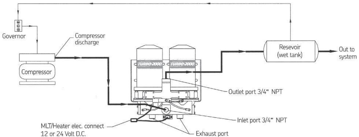
**Fig. 2** Connection schematic
