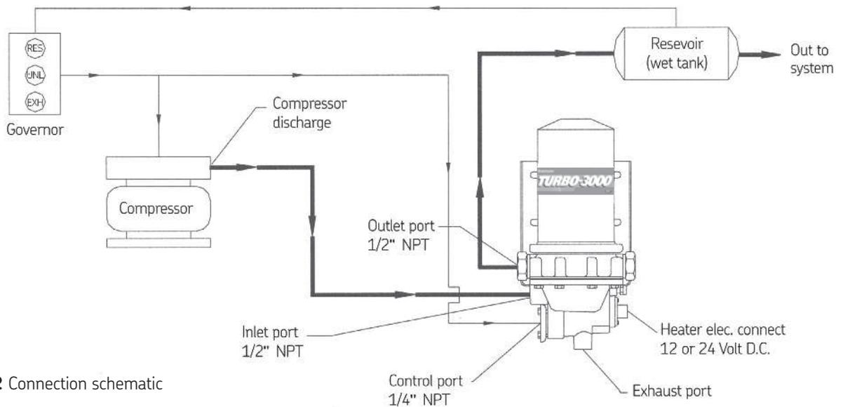
**Fig. 2** Connection schematic
