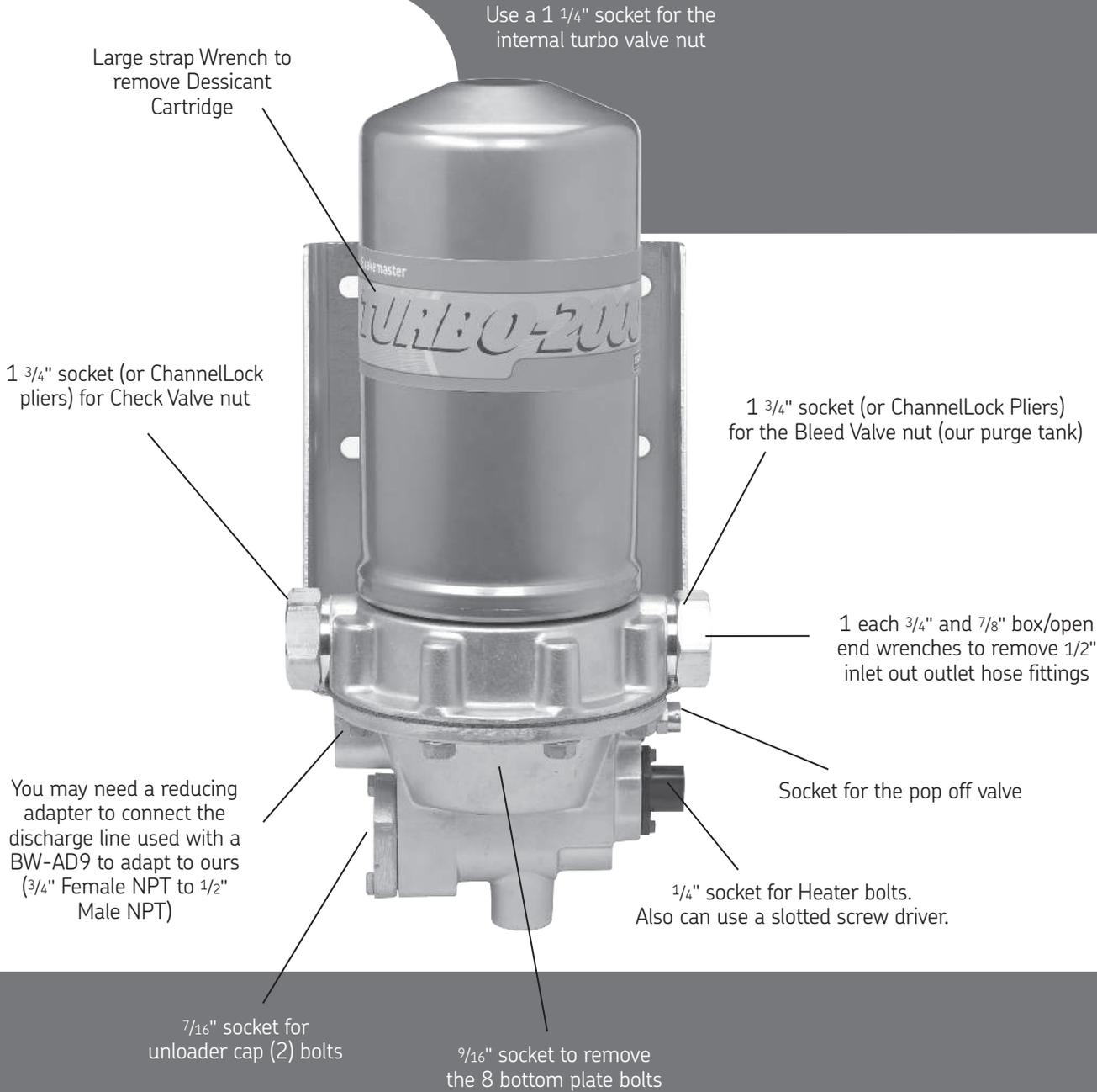
**Note: It is very difficult to remove the bottom cap bolts with a wrench. Use a socket only with a six (6) inch extension.**
